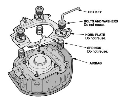
10. Install the new Horn Plate Assembly with the new bolts, washers, and springs. Torque the bolts to (3.5 ± .05 N·m), (2.5 ± .03 lb-ft).
